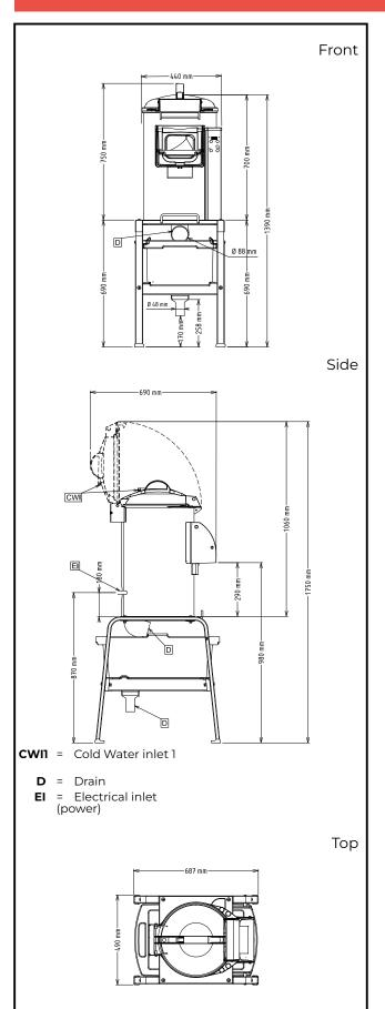
Electric Supply voltage: 603511 (DT15E1) 220-240 V/1N ph/50/60 Hz 200-240/380-440 V/3 603512 (DT15E324) ph/50/60 Hz Electrical power max.: 0.37 kW 0.37 kW **Total Watts:** Capacity: Performance (up to): 240 kg/hour Capacity: 15 litres Key Information: External dimensions, Width: 440 mm External dimensions, 690 mm Depth: External dimensions, Height: 750 mm **Shipping weight:**
